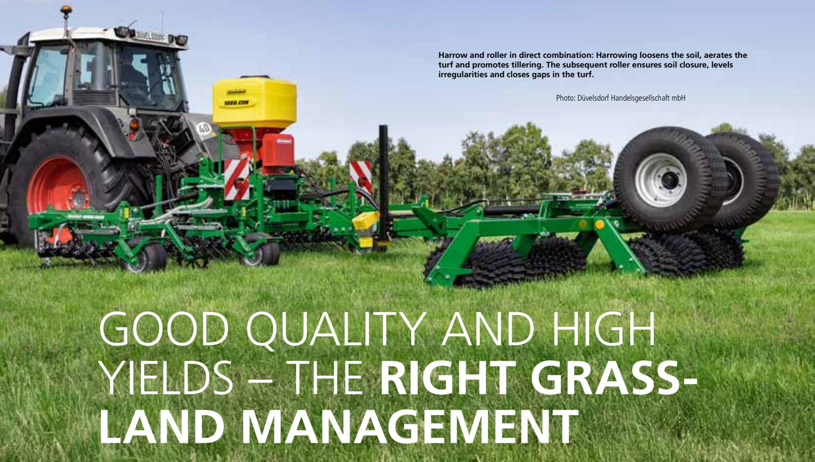
Harrow and roller in direct combination: Harrowing loosens the soil, aerates the turf and promotes tillering. The subsequent roller ensures soil closure, levels irregularities and closes gaps in the turf.
